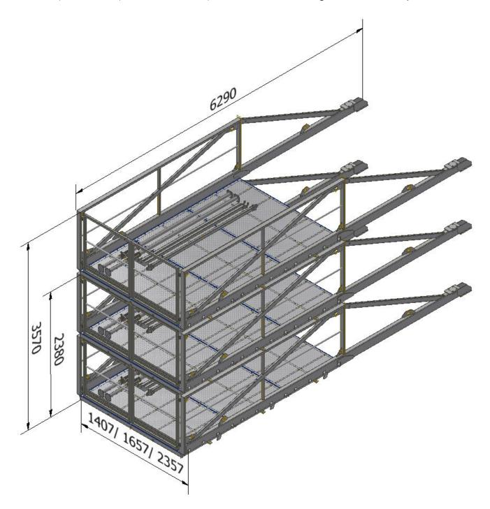
Drawing 10. Transport and storage of assembled platform
