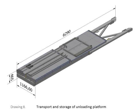
Before storing assembled platform, unfold the feet located at the bottom of the platform. The feet ensure stability while stacking.
